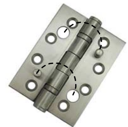
Figure 14. Lift off prevention hinges. The pin on one side will fit into the hole on the other, preventing the door from being lifted, even if the hinge pin is removed
